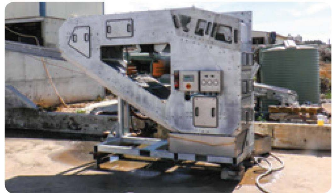
Fig 2. Z300A Z-Filter trial setup at a piggery.
