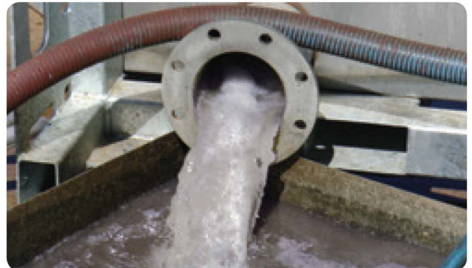
Fig 4. Filtrate being discharged from the Z300A unit.
