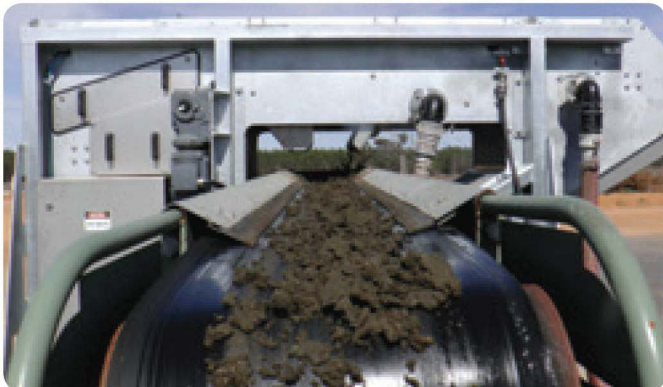
Fig 3. Solids from the Z300A being discharged onto a conveyor.
