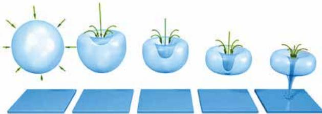
The water molecules are pulled apart by the cavitation reactions which create nano-bubbles. These help in disinfecting the water. The greater the pressure differential across a ZPM, the stronger the cavitation reactions. No energy is lost through this reaction as it is returned to the water in the form of heat.
