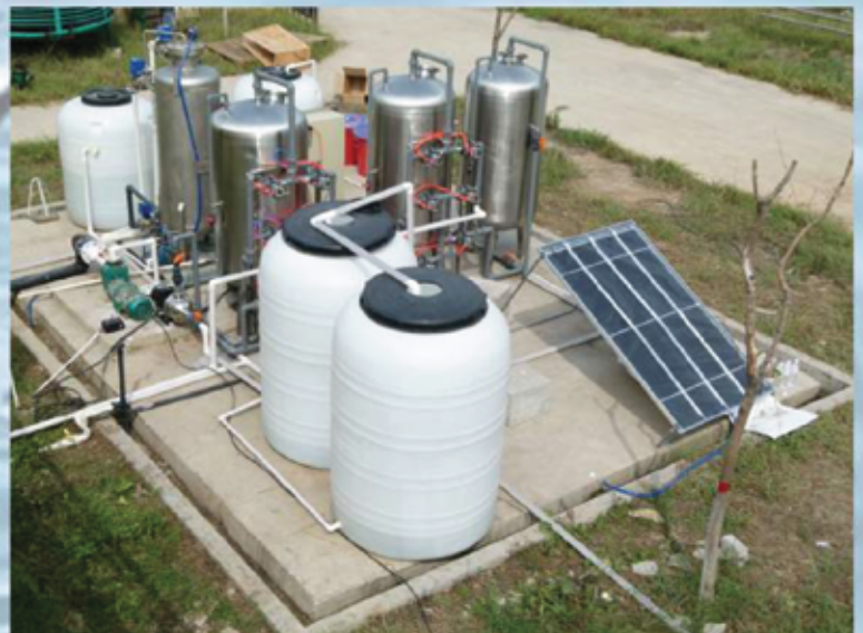
15m 3 hr with solar distillation
