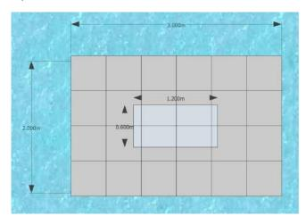
In this design the microbubble generator sits in the middle of the platform with good walkway space around it
