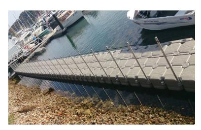
In this option, the rails are positioned every metre, positioned 500mm from each corner.
